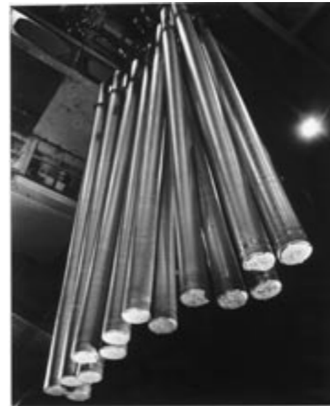
WOLFGANG SIEVERS ALUMINIUM BILLETS AFTER CASTING AT COMALCO, BELL BAY 1965 PHOTOGRAPHY 59.7 X 48.5
